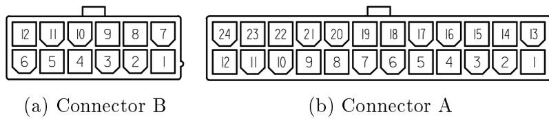
Figure 2.1: Connectors on the back of the controller and their pin numbering.
