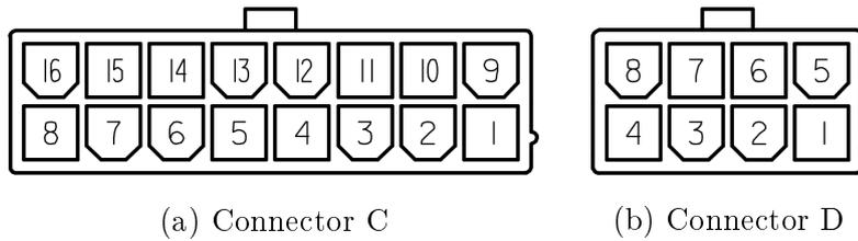
Figure B.1: Connectors on the back of the expansion board.
